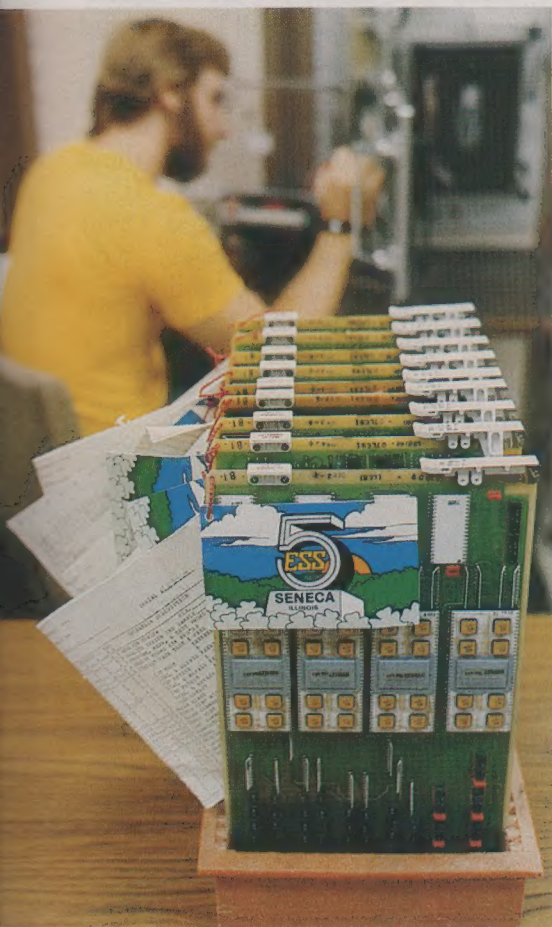
Gated diodes are vital to the operation of the No. 5 ESS. Here Tom Hankus tests Seneca's GDX boards.
